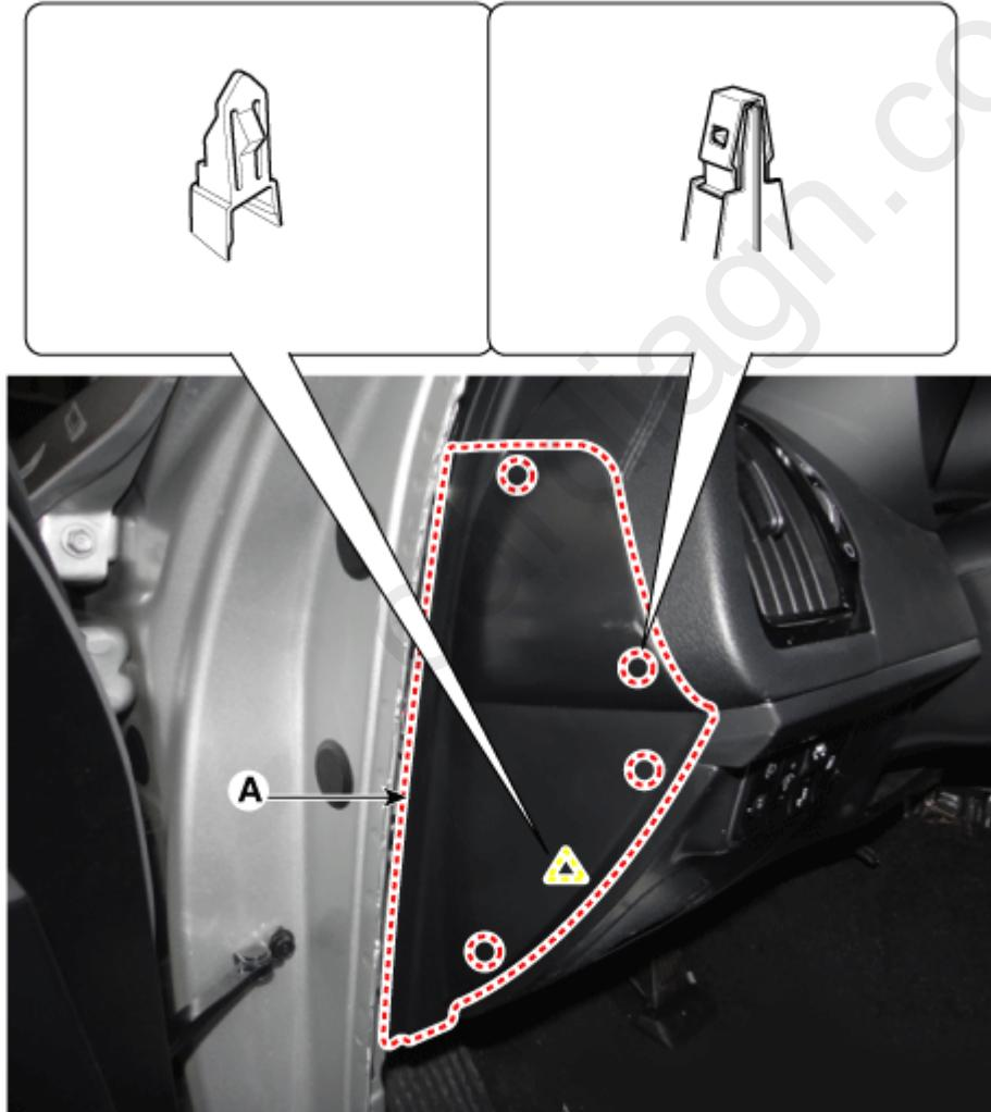
2. Separate the crash pad lower panel (A) after loosening the bolts and screws.
